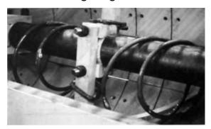
Eliminate time consuming clean-up at the end of the day's production. Cleaning rings for the shaft and arms will eliminate the build-up of material and allow longer mixing without stopping for clean-up. Arms that grow in size from material build-up also hinder proper blending of the mix. Installation instructions are included. Parts for Slump mixers include rings between arms and head liners. Additional sizes and styles are available.
