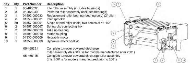
This conveyor assembly can also be retrofitted into older model turnovers to replace the slat style discharge conveyor. The assembly is designed to fit directly in place of the existing slat conveyor frame and reuse the existing hydraulic control valves and hosing.
