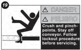
01539-400084 Crush and Pinch Hazard Width 10" Height 6"
