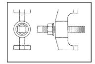
Fig. 4 - Tool 02-467006 torque to 90 ft lbs, (135 newton-meters)
