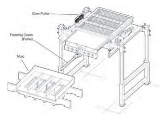
NOTE: Special hardware and software are required for your concrete products machine's electrical panel in order to control the motion of the core puller.
