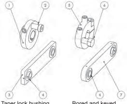
Taper lock bushing configuation
