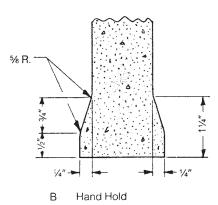
Hand hold is optional on 2 and 3 core block. Dimensions of units: In practice, the first dimension of a concrete masonry unit represents the thickness; the second dimension, the height, the third, length.
