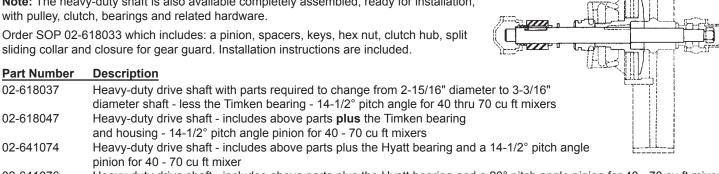
02-641076 Heavy-duty drive shaft - includes above parts plus the Hyatt bearing and a 20° pitch angle pinion for 40 - 70 cu ft mixer Parts are also available to change from the old style 2-15/16" diameter shaft (light bearing D-212) to the 2-15/16" heavy-duty shaft,
