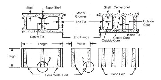
NOTE: The following nomenclature is the same for 2 core and 3 core block. The 2 core is shown here for illustration.
