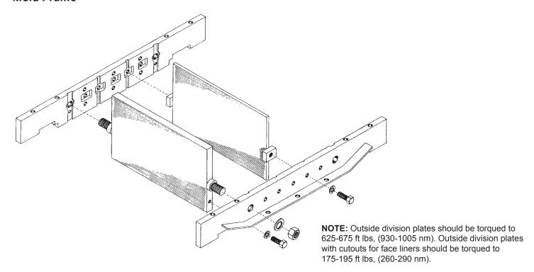
Threaded inside division plates should be torqued to 40-50 ft lbs, (60-70 nm).
