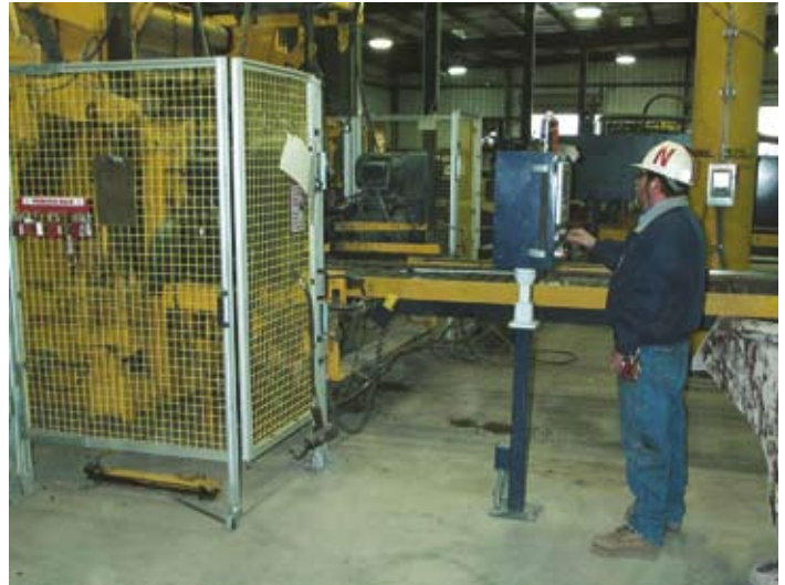
Rolling swing-out fencing provides access to the concrete products machine for mold changes and adjustments while providing necessary guarding during machine operation.
