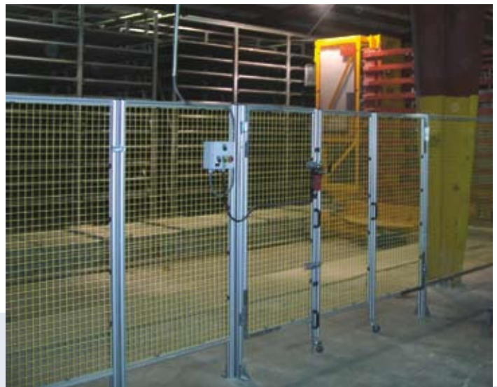
The access gate to the kiln area is equipped with an entry box which brings the finger car to a safe, controlled stop before unlocking.
