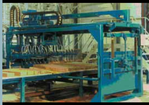
A washing machine cleans the surface of pavers and kerbs after they leave the concrete products machine.
