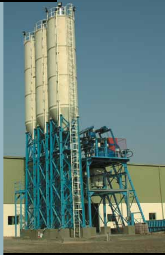
Concrete mixing plant.
